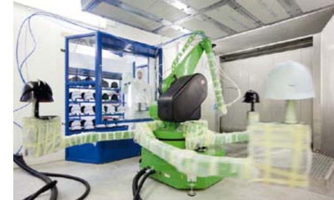
One a minute: A five-armed coating robot applies one of seven colors to the helmet.
