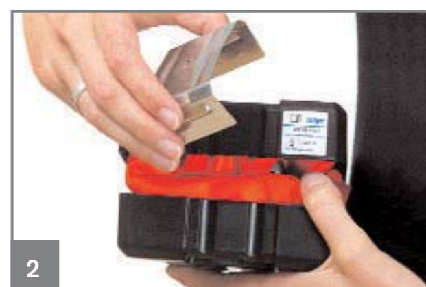
2 Remove the metal clamp to open the box and remove the hood.
